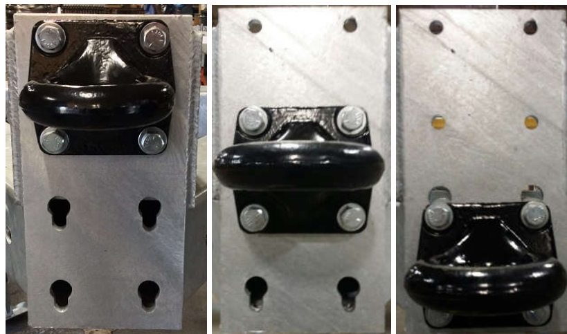
Figure 6. Mounting Positions of Lunette Ring
